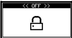
Image displayed when switched to off. When set to OFF, the engine cannot be started in any way and, if it is running, it stops without the engine cooling step.
