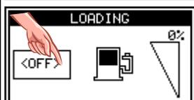
Filling OFF: turns filling off; the output, if enabled, is disabled.
