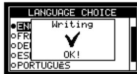
The chosen parameter is now programmed in the control unit. The settings are stored in a non-volatile memory, and are therefore maintained even if the power is switched off. The value can be modified at any time by repeating the procedure as described above.
