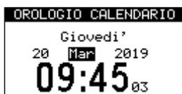
The value shown can be changed using the UP\_BUTTON or DOWN\_BUTTON. To change selection, use the RIGHT\_BUTTON or the LEFT\_BUTTON. To exit settings, use the TORTOISE\_BUTTON or press the START\_STOP\_BUTTON. It does not require confirmation. The time is retained by the control unit even when it is not powered, thanks to an internal battery. If the internal battery is not installed, the following date and time will appear on start-up: 1/01/2019, 00:00.00.
