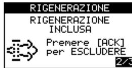
During regeneration, the engine ECU sends the necessary signals, displayed in the instrument LAMPS
