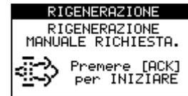
The Stationary regeneration can be interrupted by deactivating the parking switch, turning the engine off, or disabling the regeneration just like for the Reset regeneration.
