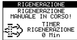
To interrupt the Standstill regeneration, set the parking switch on OPEN.
