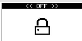
Image displayed when switched to off. When set to OFF, the engine cannot be started in any way and, if it is running, it stops without the engine cooling step.
