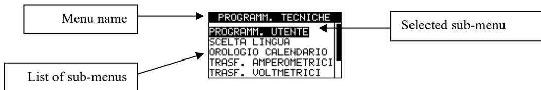
Press the two **UP** and **DOWN** buttons to scroll through the programming sub-menus. Press **RIGHT** to enter a sub-menu. For example:
