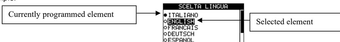
Press the two **UP** and **DOWN** buttons to scroll through the programming items. For example:
