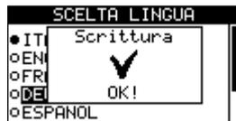
The chosen parameter is now programmed in the control unit. The settings are stored in a non-volatile memory, and are therefore maintained even if the power is switched off. The value can be modified at any time by repeating the procedure as described above.
