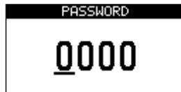
The control unit requires a password. The factory password 7 (DEVICE) is "2015" and all the others are "0000"; these can be changed by the user. Use the **ARROW** buttons to enter the code. Then press **START** to confirm the password and access the technical programming menus.
